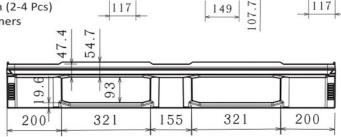
All dimensions may vary ±5 mm due to the production process & raw material characteristics.
