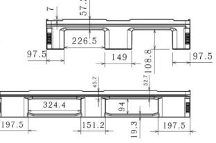
All dimensions may vary ±5 mm due to the production process & raw material characteristics.
